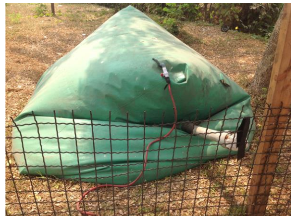
Figure 3: Production of biogas in a partially buried balloon (at ISTA Ndolo, Barumbu municipality)
