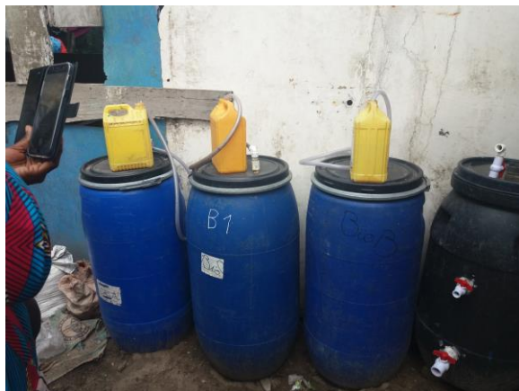
Figure 2: Biogas production in 220 liter plastic containers (at Green Space Network in Kingabwa, Limete municipality)
